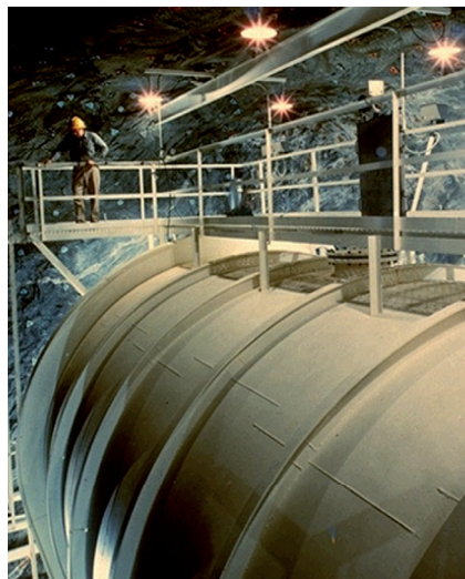
Figure 2: The Homestake solar neutrino detector
